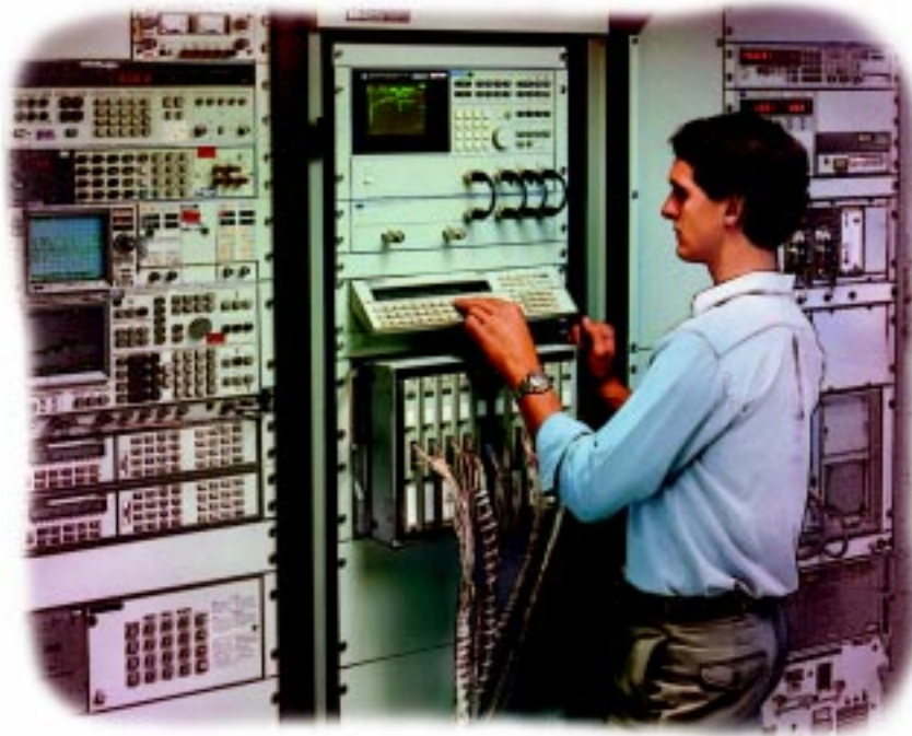
IEEE-488 has been the industry standard interface for connecting instruments to computers for automating measurements.
